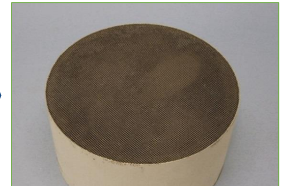
Coating of a full size NSC demonstrator
